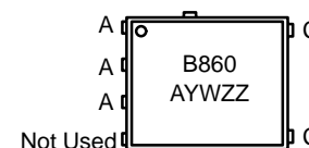
SO-8 FLAT LEAD CASE 488AA STYLE 2
