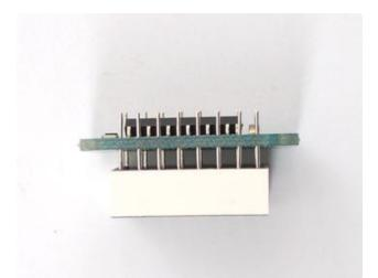
Remove the parts from packaging and place the LED matrix OVER the silkscreen side. It can go 'either way' - the matrix is symmetric so as long as it goes onto the front it will work in any orientation. Do not solder the matrix over the chip on the back of the backpack - it will not work then!
