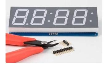
Cut the header strip to length if necessary and insert LONG pins down into the breadboard.
