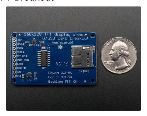
This color display uses SPI to receive image data. That means you need at least 4 pins - clock, data in, tft cs and d/c. If you'd like to have SD card usage too, add another 2 pins - data out and card cs. However, there's a couple other pins you may want to use, lets go thru them all!
