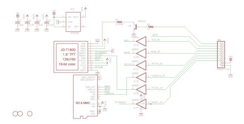
For the level shifter we use the CD74HC4050 which has a typical propagation delay of  $^{\sim}10 \text{ns}$
