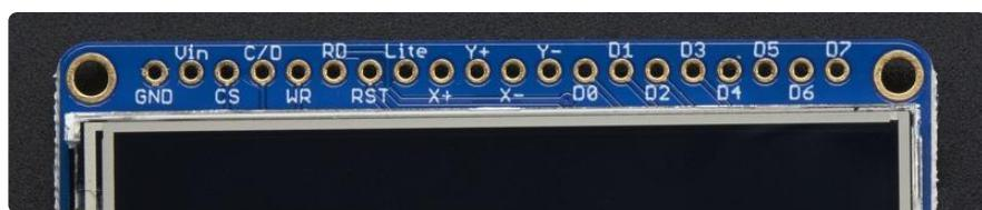
Make sure you're soldering and connecting to the 8-bit side!
