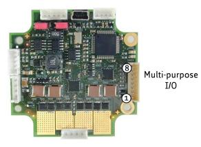
Figure 3.2 I/O connector
