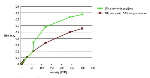
Figure 1.2 Energy efficiency example with coolStep
