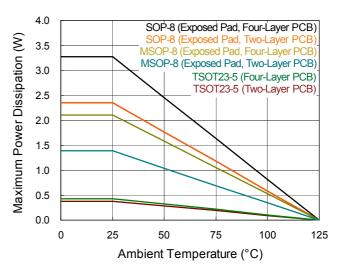
Figure 2. Derating Curves of Maximum Power Dissipation
