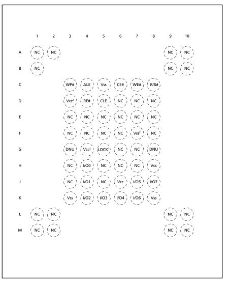
Notes: 1. For the 3V device, G5 changes to DNU. NO LOCK function is available on the 3.3V device.
