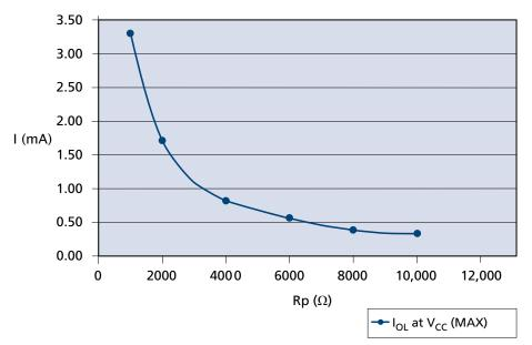
Figure 21: I<sub>OL</sub> vs. Rp (1.8V V<sub>CC</sub>)
