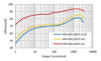
Figure 3. Efficiency vs Load Current, Vin=36V
