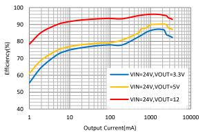
Figure 4. Efficiency vs Load Current, Vin=24V
