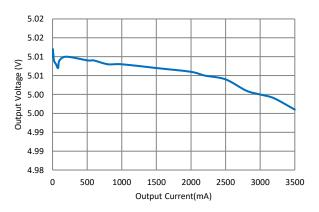
Figure 6. Load Regulation (Vout=5V)
