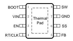
Figure 2. 8-Lead Plastic E-SOP
