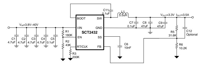
Figure 19. SCT2432 Design Example, 3.3V Output with Programmable UVLO
