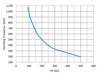
Figure 8.Clock Frequency vs RT/CLK Resistor
