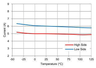
Figure 14. Peak Current Limit vs Temperature
