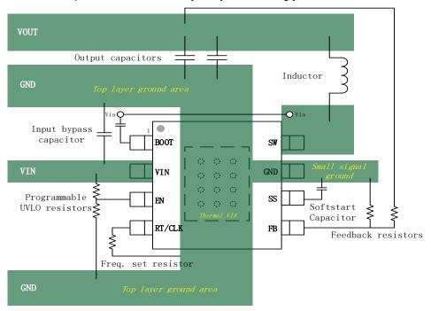
Figure 26. PCB Layout Example
