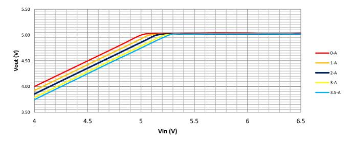
Figure 18. LDO Operation Characteristic (Vout =5V)
