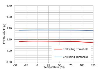
Figure 11. EN Threshold vs Temperature
