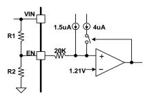
Figure 16. System UVLO by enable divide
