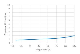
Figure 9. Shutdown Current vs Temperature
