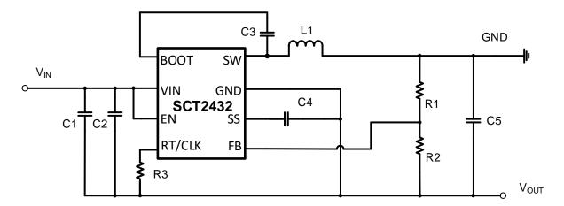
Figure 20. SCT2432 Inverting Power Supply
