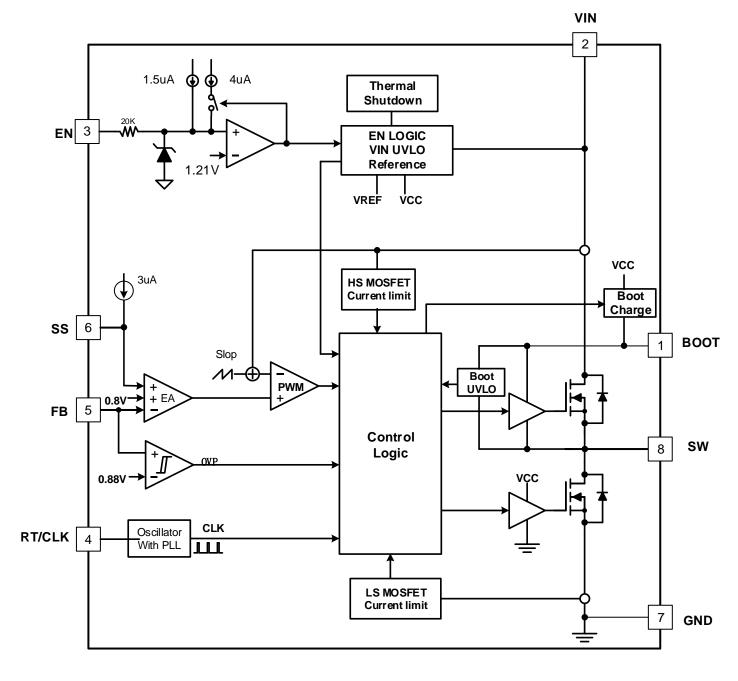
Figure 15. Functional Block Diagram
