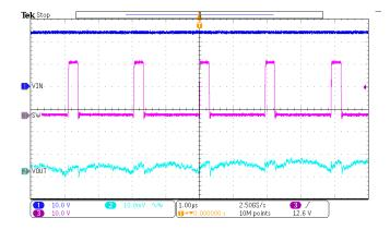
Figure 25. SW and Vout Ripple
