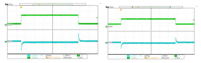
Figure 23.Load Transient (0.35A-3.15A, 250mA/us)
