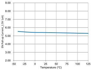
Figure 12. EN Pull-up Current vs Temperature
