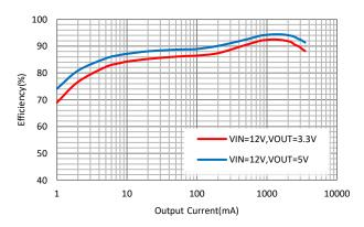
Figure 5. Efficiency vs Load Current, Vin=12V
