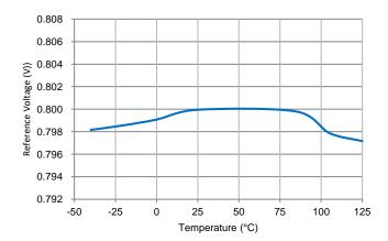
Figure 13. Reference Voltage vs Temperature
