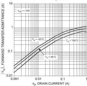
Fig. 19 Forward Transfer Admittance vs. Drain Current
