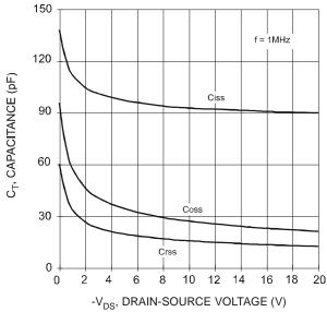
Fig. 20 Typical Capacitance
