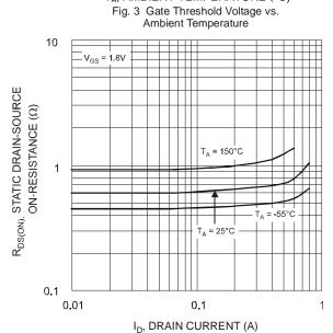
Fig. 5 Static Drain-Source On-Resistance vs.
