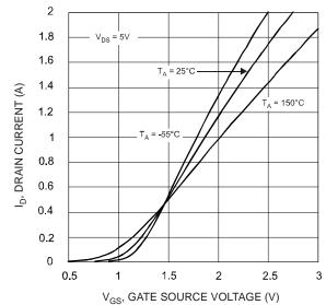
Fig. 2 Typical Transfer Characteristics
