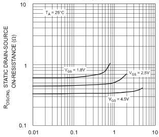
I<sub>D</sub>, DRAIN-SOURCE CURRENT (A) Fig. 6 Static Drain-Source On-Resistance vs. Drain-Source Current vs. Gate Source Voltage
