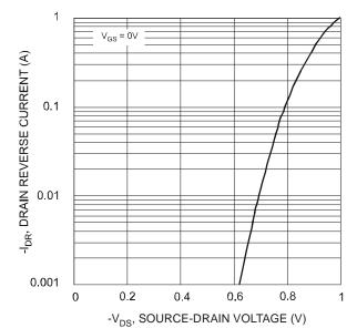
Fig. 18 Reverse Drain Current vs. Source-Drain Voltage
