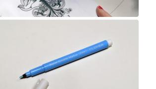
Use a water-disolvable marker to plan out your circuit traces.
