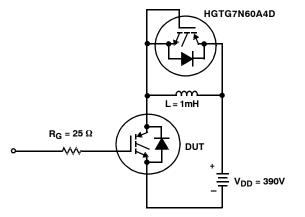
Figure 24. INDUCTIVE SWITCHING TEST CIRCUIT
