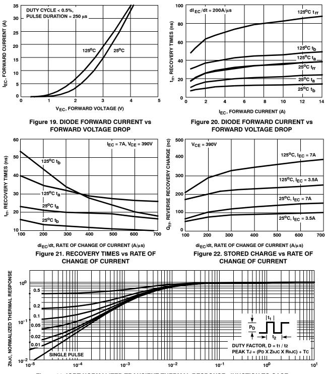
Figure 23. IGBT NORMALIZED TRANSIENT THERMAL RESPONSE, JUNCTION TO CASE
