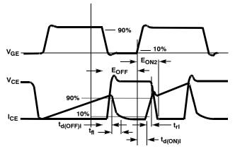
Figure 25. SWITCHING TEST WAVEFORMS
