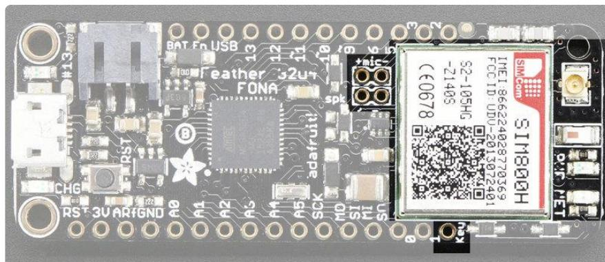
Now to the fun part, the cellular module. There's a few pins that are used to control the module. It uses SoftwareSerial to communicate with the microcontroller
