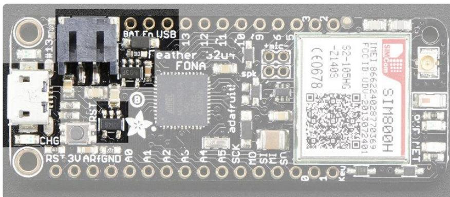
The above shows the Micro USB jack (left), Lipoly JST jack (top left), as well as the 3.3V regulator and changeover diode (just to the right of the JST jack) and the Lipoly charging circuitry (to the right of the Reset button). There's also a CHG LED, which will light up while the battery is charging. This LED might also flicker if the battery is not connected or when the cellular module is in action
