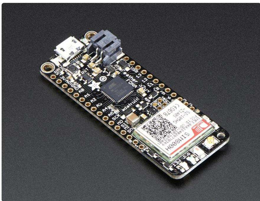
At the Feather 32u4's heart is an ATmega32u4 clocked at 8 MHz and at 3.3V logic, a chip setup we've had tons of experience with as [it's the same as the Flora](https://adafru.it/dVl) (<https://adafru.it/dVl>). This chip has 32K of flash and 2K of RAM, with built in USB so not only does it have a USB-to-Serial program & debug capability built in with no need for an FTDI-like chip, it can also act like a mouse, keyboard, USB MIDI device, etc.
