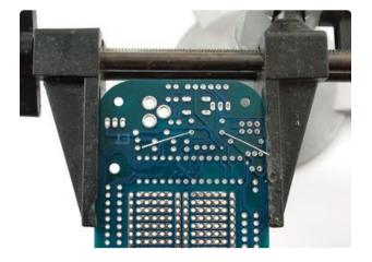
Bend out the long metal leads so the resistor sits flat agains the board, and flip the PCB over.
