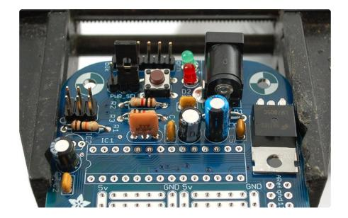
Make sure that the green LED is lit once you have the board powered, if the green LED is off, there's no power - check your adapter or battery or cable and get the LED lit before continuing.
