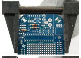
R2 is used to set the brightness of the green LED, which indicates when the board is correctly powered.
