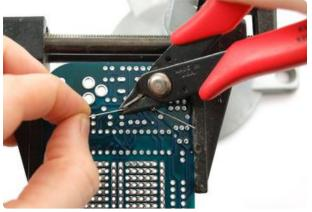
Using your diagonal cutters, cut off the long leads just above the solder joint.
