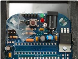
Place one piece of the header, the 6-pin piece, into the spot right next to the green LED. Make sure the short legs are sticking down into the PCB and the long legs are sticking up. This is the programming header. This is where you can connect an FTDI cable or FTDI friend to reprogram the Menta.
