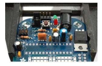
Finally you can place the jumper into the PWR\_SEL spot. For now, place it on the right hand side, in the DC position - this indicates that you'll be powering it via the big DC jack.
