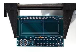
We'll start with the first resistor R1 - which has yellow, violet, red, gold bands on it. This resistor is part of the interface between the Arduino and the 'port expander' that controls the LCD.
