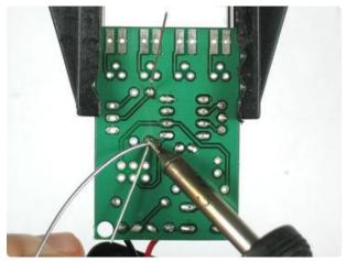
Solder and clip the resistor.
