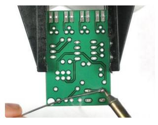
Using your soldering iron, heat up a leg of the button and the poke solder into it to make a nice solder joint.
