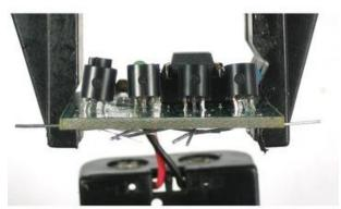
Next are the four NPN (2N2222) transistors Q1 Q2 Q3 and Q4. These are the devices that turn on and off the high power IR LEDs. The microcontroller doesn't have the capability to provide a lot of power directly to the LEDs so these transistors assist it.
