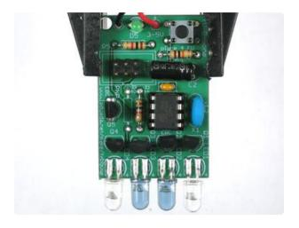
If you're planning to reprogram the chip, solder in the 6-pin ICSP header. The long pins go up.
