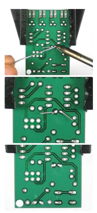
Solder and clip the ceramic capacitor part.
