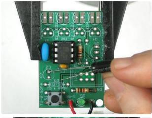
Next is the 220uF electrolytic capacitor. It is polarized so make sure it goes in the right way. The long lead is positive, and goes into the hole marked with a +, on the right in this photo.
