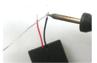
Use your soldering iron to 'tin' the wire, melting solder into it to keep the wire from fraying.
