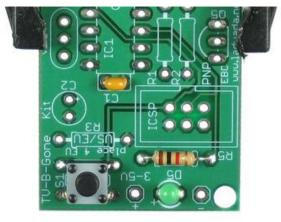
The next part is the ceramic capacitor C1. Ceramic capacitors are symmetric so it can go in either way.
