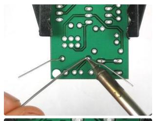
Solder each leg of the resistor.
