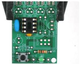
Next, place 2 components. The ceramic oscillator and the 8-pin socket. The oscillator has 3 pins and is symmeteric. The oscillator is the timeclock for the microcontroller, making sure that it is performing its functions at the correct speed.
