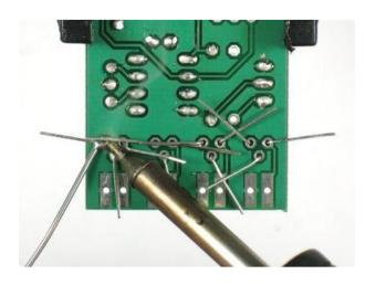
Turn the PCB over and solder in all the transistors. Then clip the wires.
