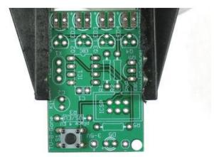
The first part we're going to assemble is the button. The button is a symmetric part so it can go in two ways. Line up the metal legs with the holes in the circuit board and snap it in. The button should sit flat against the circuit board.
