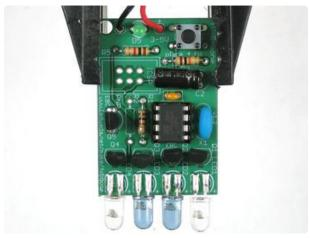
If you're in the EU, UK, Australia, place the remaining 10K resistor into R3. This will tell the micrcontroller to use the EU database.
