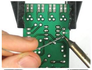
Solder the rest of the points then clip short the legs of the oscillator.
