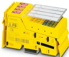
Safety-related digital output module, IP20 degree of protection, for SafetyBridge, INTERBUS-Safety, and PROFIsafe systems. The module has four safe digital outputs for two-channel assignment or eight safe digital outputs for single-channel assignment
