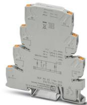
Terminal block for filtering test pulses from safe semiconductor outputs with adjustable filter values (1.5  $\mu$ F/11.5  $\mu$ F), as well as for EMC filtering of 24 V signals up to an amperage of 2 A.
