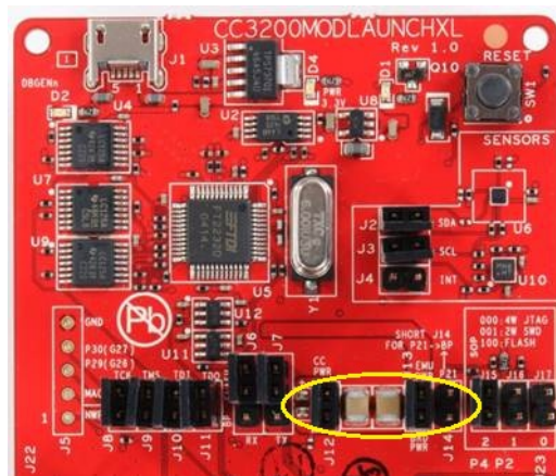
Figure 9. Powering From USB
