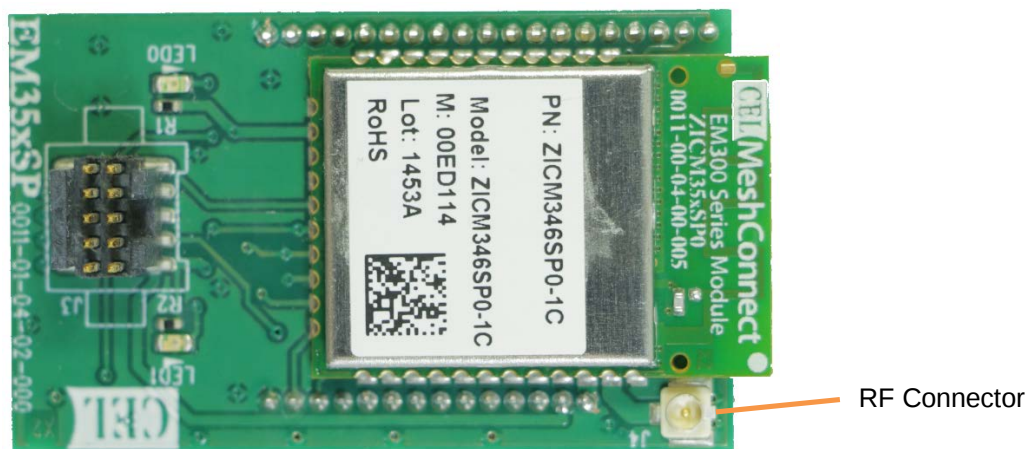
Figure 17. Module with U.FL RF Connector
