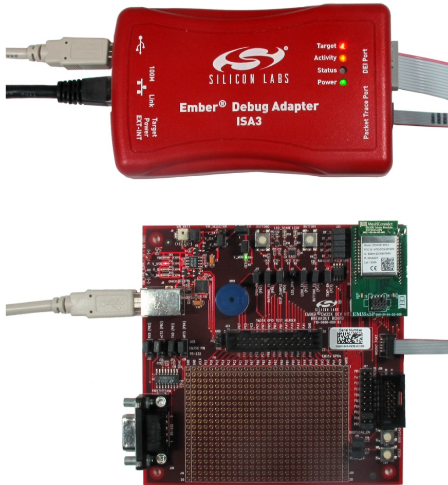
Figure 15. Ember Debug Adapter (ISA3) Supplying Power; FTDI Serial <-> USB Converter Used for Communication
