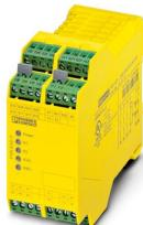
Safety relay for emergency stop and safety door monitoring up to SIL 3 or Cat. 4, PL e in accordance with EN ISO 13849, automatic or manual activation, 3 N/O contacts, 1 N/C contact, 2 N/O contacts with a fixed dropout delay of 2 s, plug-in screw connection terminal blocks
