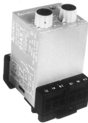
The DIAR.T is a current control which is capable of sensing up to 100 Amps. If requires a stepdown transformer, T1 100. The transformer has a 0.4" diameter center hole through which a current carrying lead is routed. Automatic or manual unlatching is available in each unit.
