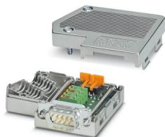
D-SUB plug, 9-pos., pin, axial version with two 35° cable entries, bus system: PROFIBUS DP up to 12 Mbps, termination resistor can be switched on via slide switch, pin assignment: 3, 5, 6, 8; spring-cage connection terminal blocks
