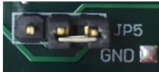
Figure 2B. (JP5: Pin 2 - 3 to Banana Jack)
