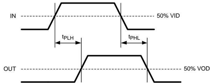
**Figure 2. Propagation Delay From Input to Output**
