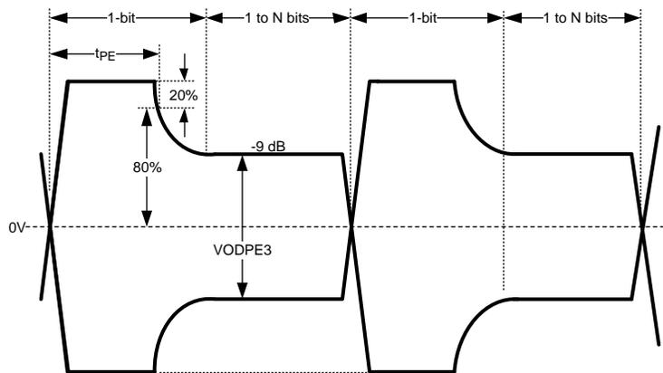
**Figure 3. Test Condition for Output Pre-Emphasis Duration**
