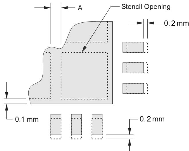
Figure 18. No Pullback WQFN, Single Row Reference Diagram
