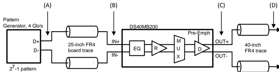
Figure 11. Block Diagram of DS40MB200 Application Example
