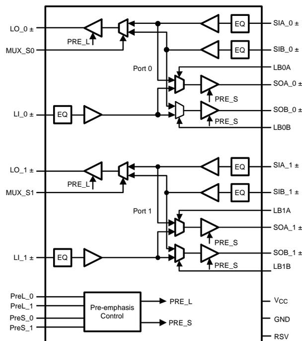
All CML inputs and outputs must be AC coupled for optimal performance.
