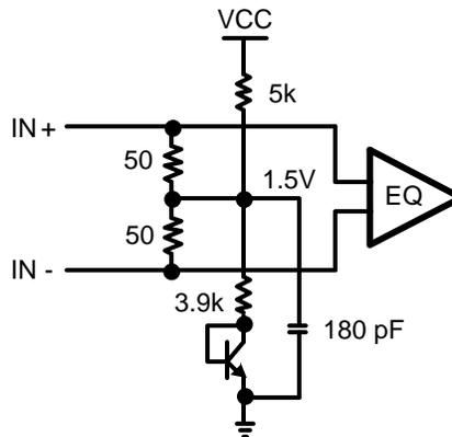
Figure 7. Receiver Input Termination and Bias Circuit
