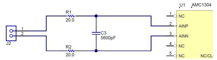
Figure 3-1. AMC1304EVM Schematic: Analog Input Section
