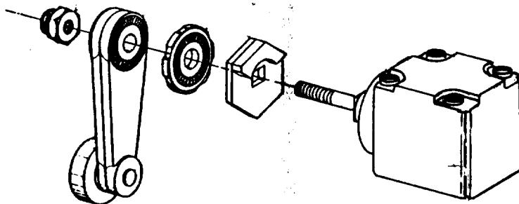
ADJUSTABLE TO OPERATE CLOCKWISE, COUNTER-CLOCKWISE, OR IN BOTH DIRECTIONS.
