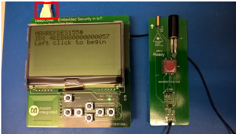
Figure 7. Power the MAX32600MBED# and MAXREFDES155# using the DEV USB port.
