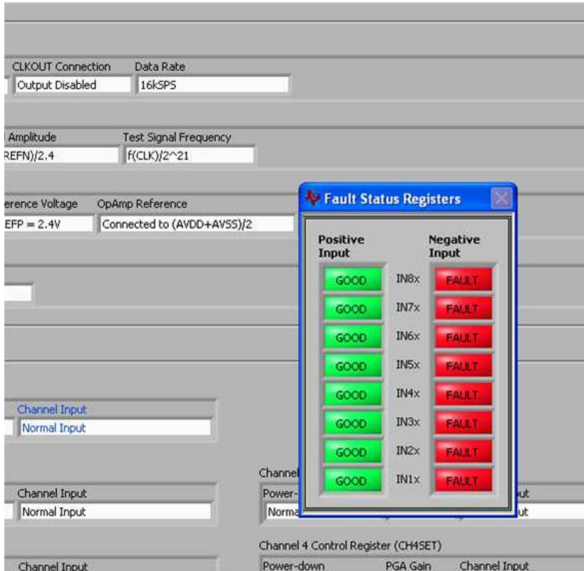
Figure 20. Fault Status Indicator
