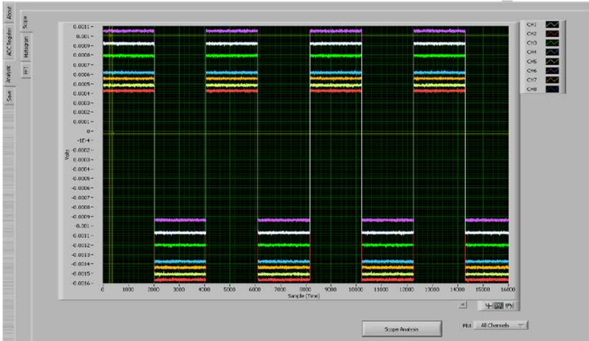
Figure 16. Example of Internal Test Signals Viewed on the Scope Display Tab
