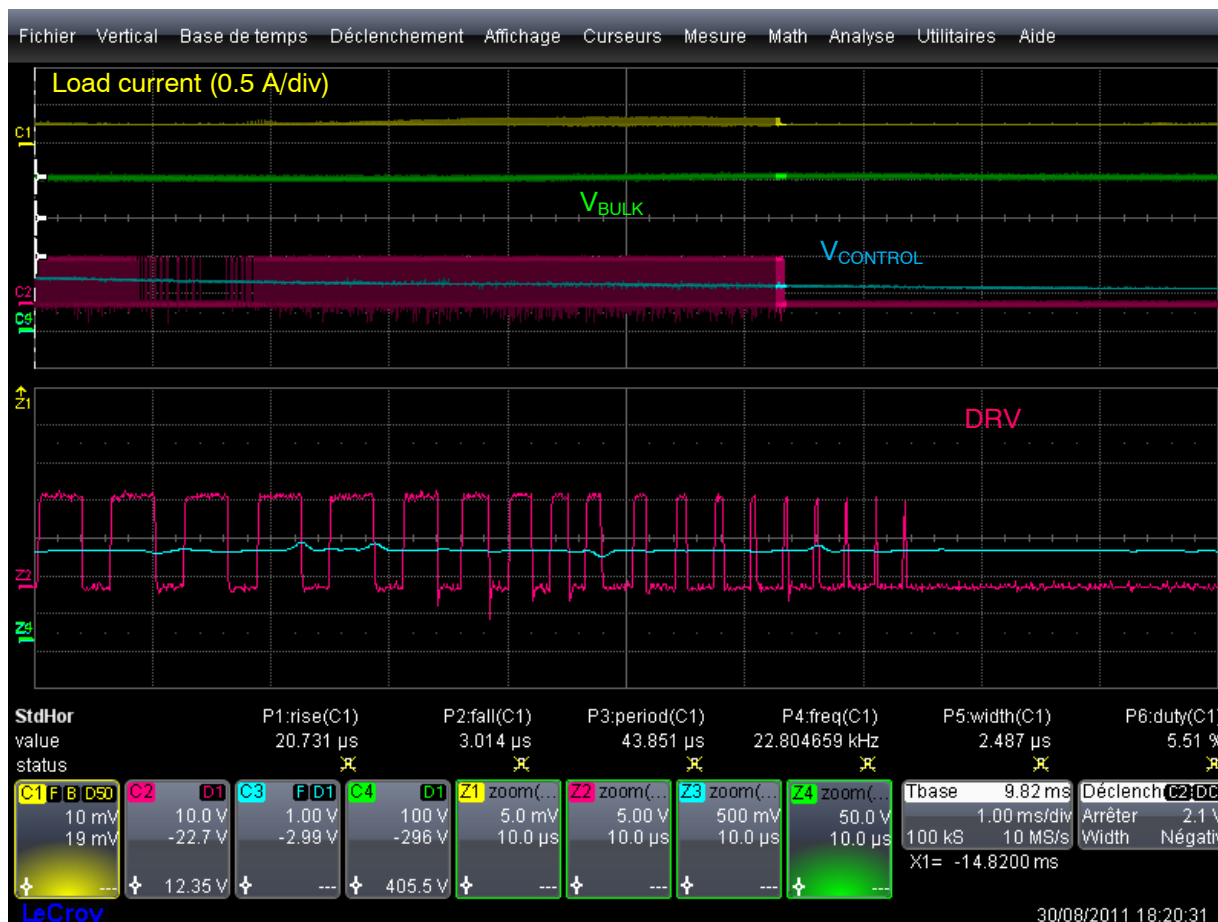
Figure 16. Soft Over-Voltage Protection
