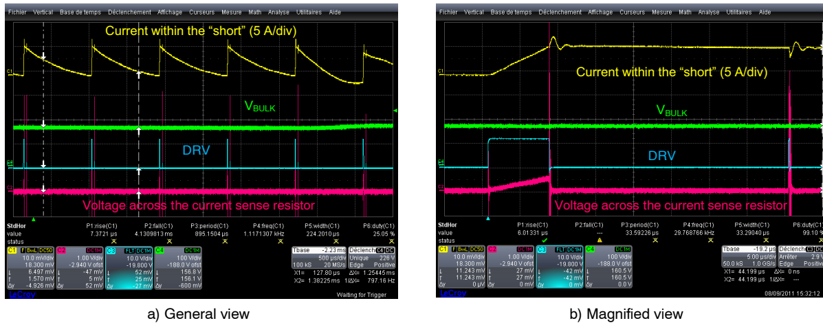
Figure 18. Shorting the Bypass Diode and the NTC
