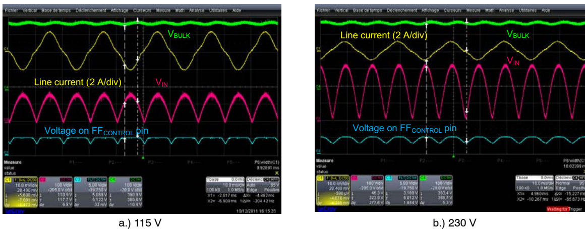
Figure 4. General Waveforms at Full Load
