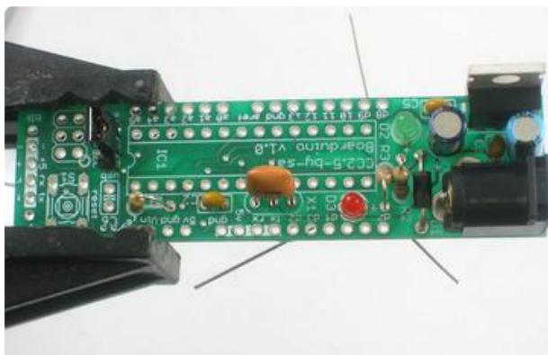
Place the red LED D3, taking care to make sure the long lead is in the positive-marked hole. Also place the matching 1K resistor R3
