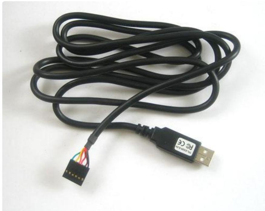
The easiest way to start loading Arduino sketches into the DC Boarduino is to use a FTDI USB cable. These cables have the USB chip inside the cable and a 6-pin socket on the end.
