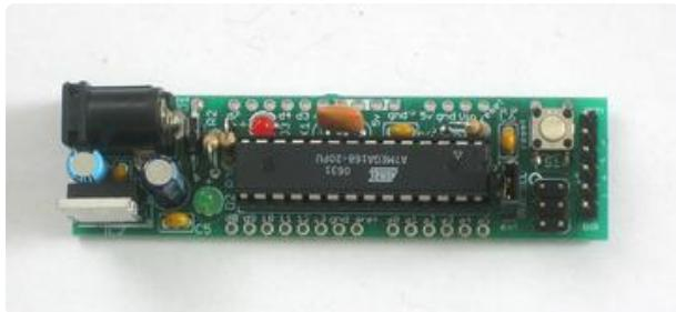
If you'd like to take advantage of the auto-reset capabilities added to the Arduino software, install ceramic capacitor C6.
