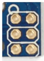
If you want to use the chip as a non-Arduino, rather you just want it as an AVR devboard, you can reprogram it via the ISP port. We provide a 2x3 pin standard ISP header. Pin 1 is indicated with a circle.
