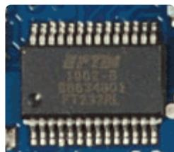
The serial converter is soldered on board, it is a FT232RL. It works great as a USB/serial chip. There are two LEDs connected to it, labeled RX and TX which will blink when data is received or transmitted. A capacitor between the DTR pin and the AVR's Reset pin acts as the auto-reset for reprogramming, which is standard on all classic Arduinos.
