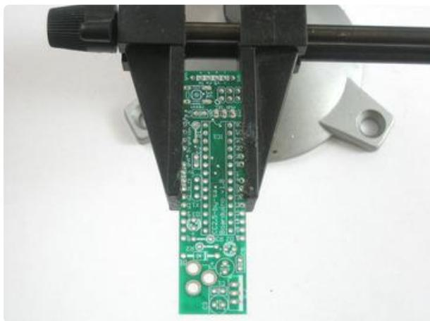
Place the PCB in a vise to make soldering easy!
