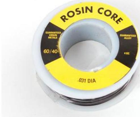
You will want rosin core, 60/40 solder. Good solder is a good thing. Bad solder leads to bridging and cold solder joints which can be tough to find.
