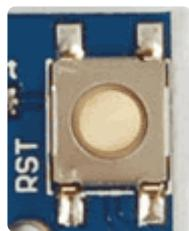
There is a single button that you can press to reset the board, the board has the Arduino bootloader auto-reset capability so you don't need to press this before uploading.
