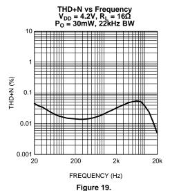
THD+N vs Frequency  $V_{DD}$  = 4.2V,  $R_L$  = 32 $\Omega$   $P_O$  = 30mW, 22kHz BW
