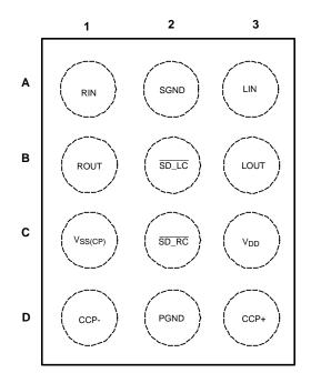
Figure 2. DSBGA - Top View See YZR0012 Package
