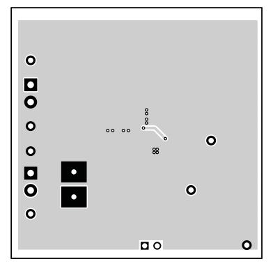
Figure 20. TPS54062EVM-695 Bottom-Side Assembly
