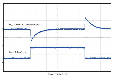
Figure 5. TPS54062EVM-695 Load Transient Response
