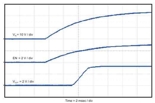
Figure 14. TPS54062EVM-695 Start-Up Relative to V<sub>IN</sub>
