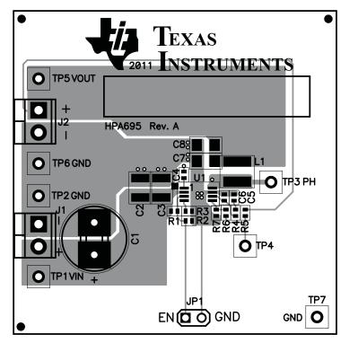
Figure 18. TPS54062EVM-695 Top-Assembly Layout
