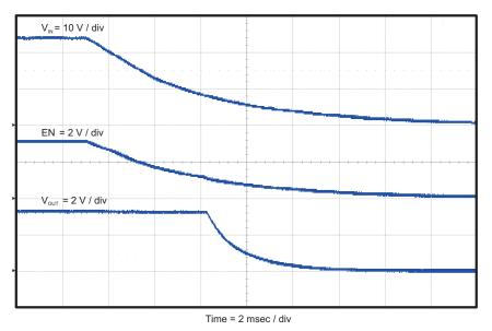
Figure 16. TPS54062EVM-695 Shutdown Relative to V<sub>IN</sub>
