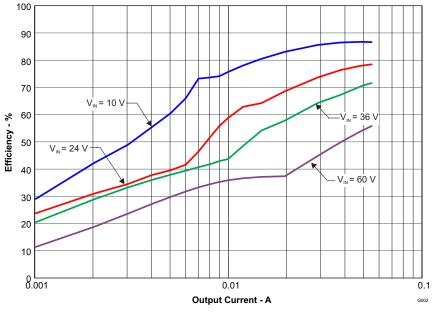
Figure 2. TPS54062EVM-695 Low Current Efficiency
