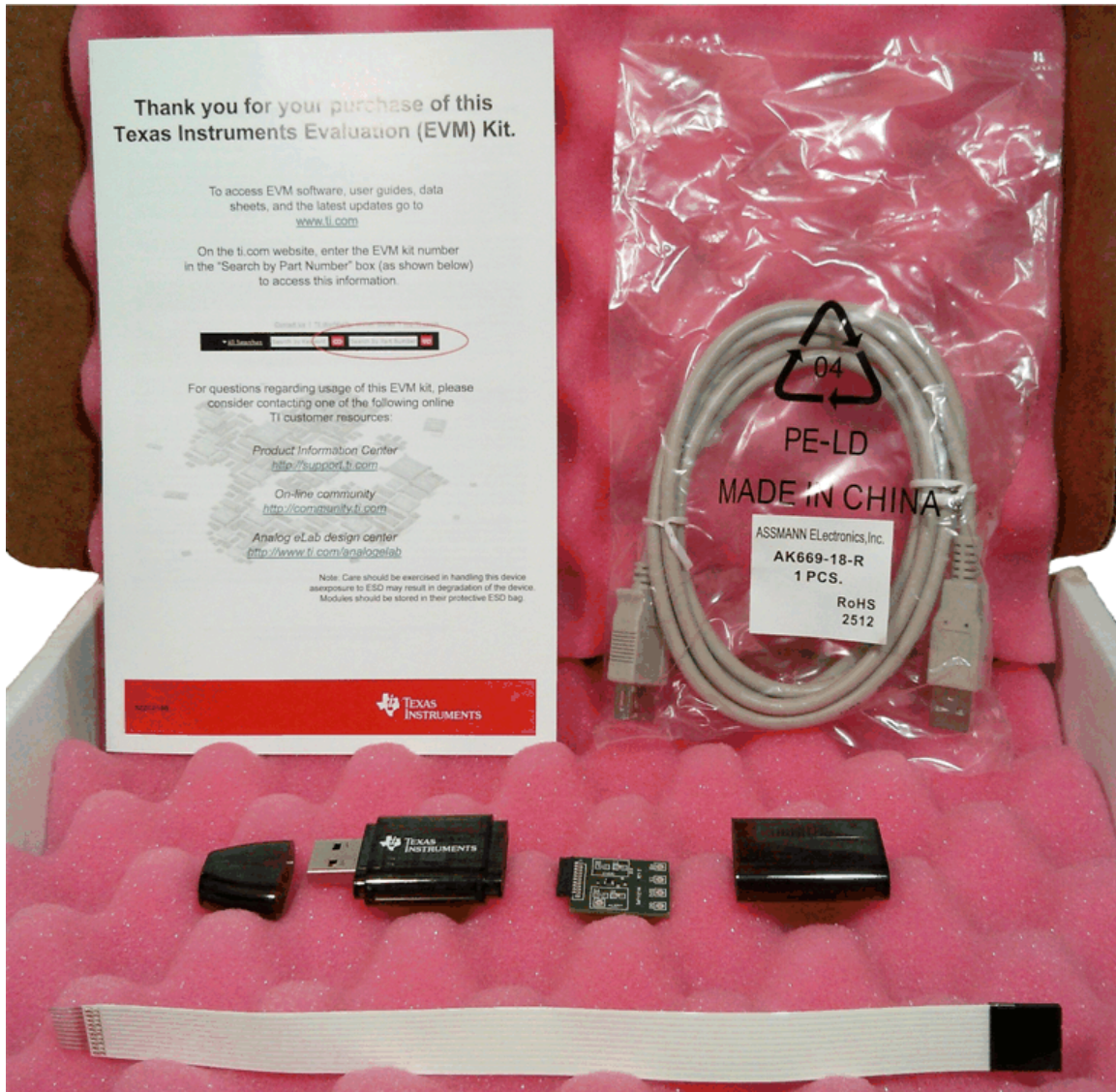
Figure 1. Hardware Included with TMP112EVM Kit
