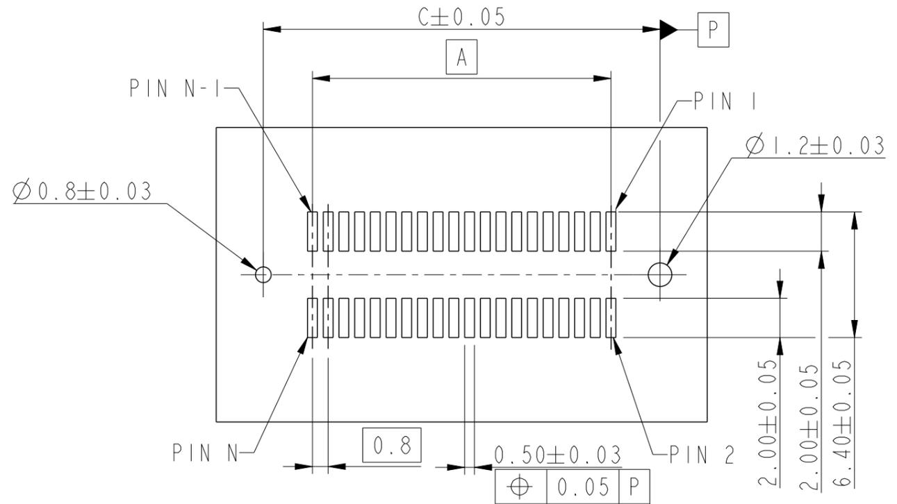
RECOMMENDED PCB LAYOUT WITH PEGS
