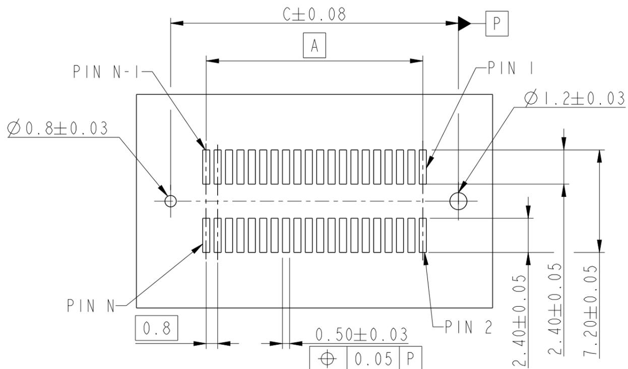
RECOMMENDED PCB LAYOUT WITH PEGS
