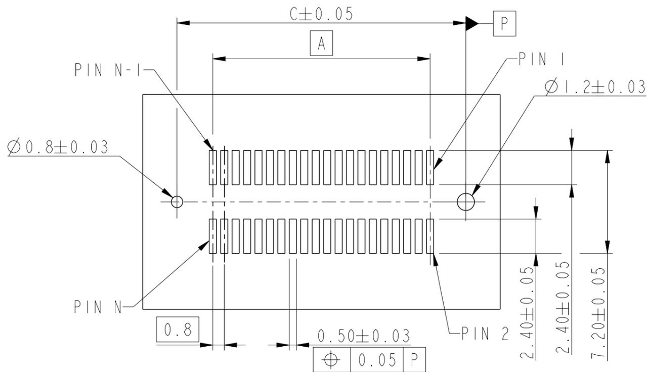
RECOMMENDED PCB LAYOUT WITH PEGS
