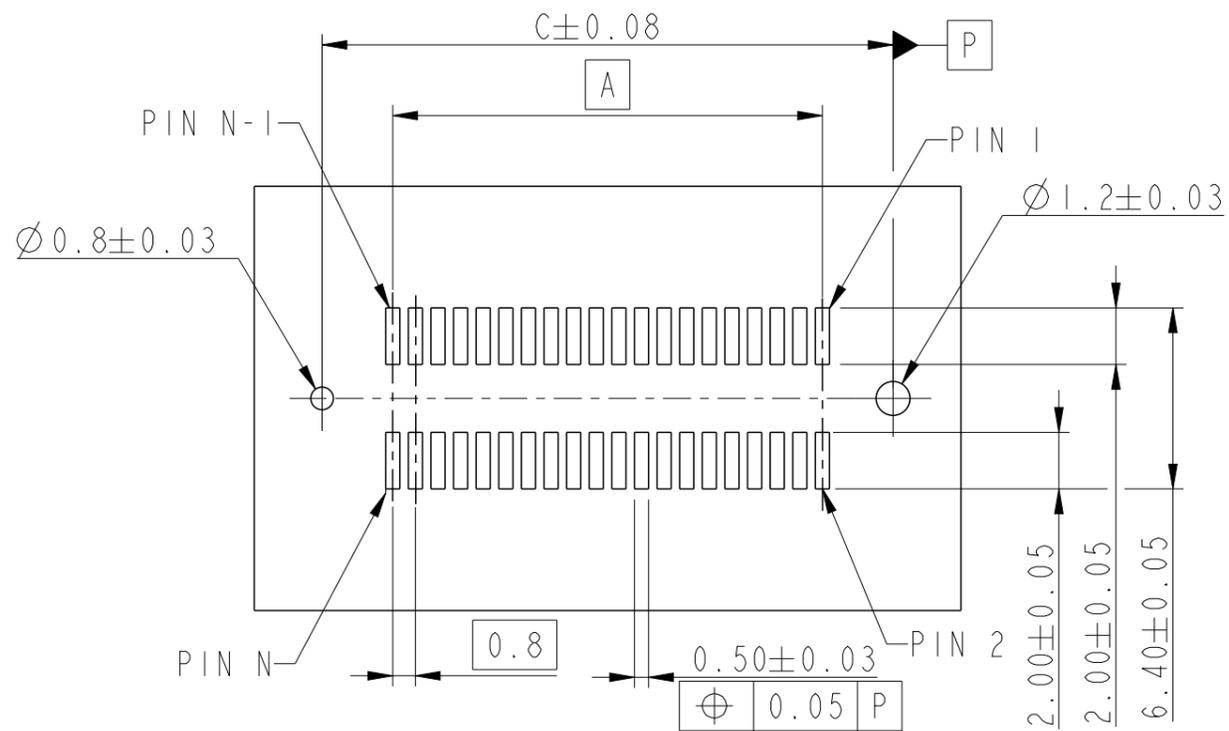
RECOMMENDED PCB LAYOUT WITH PEGS
