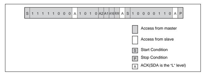
Even if the MB85RC1MT stays in the Sleep mode, SDA and SCL signals are monitored. Following sequences enable the transition to Standby mode after recovery time (tree) of internal regulator circuits.
