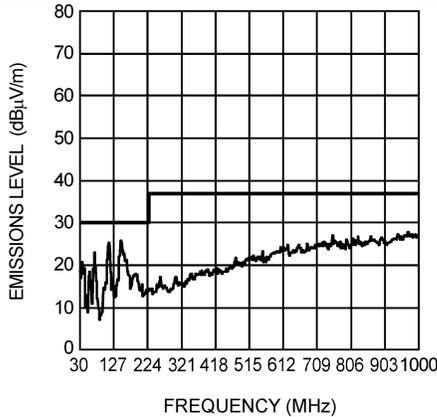
Figure 9. Radiated Emissions (EN 55022, Class B)
