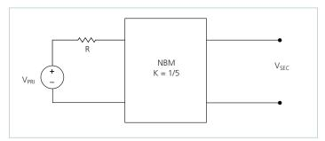
Figure 20 — K = 1/5 NBM with series primary resistor
