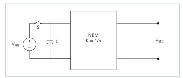
Figure 21 — NBM with primary capacitor
