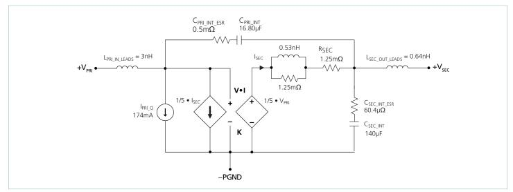
Figure 19 — NBM AC model
