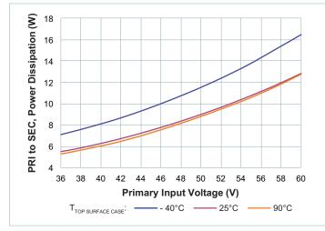
Figure 4 — No load power dissipation vs. V<sub>PRI DC</sub>
