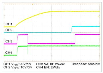
**Figure 17** — Start up from application of  $V_{PRI\_DC} = 54V$ , 20%  $I_{SEC\ OUT\ DC}$ , 100%  $C_{SEC\ OUT\ EXT}$
