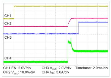
**Figure 18** — Start up from application of EN with pre-applied  $V_{PRI\_DC} = 54V$ , 20%  $I_{SEC\_OUT\_DC}$ , 100%  $C_{SEC\_OUT\_EXT}$
