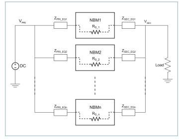
Figure 25 — NBM parallel array
