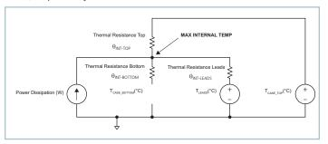
Figure 23 — Top case and leads thermal model
