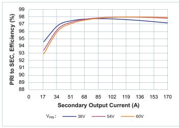
**Figure 6** — Efficiency at  $T_{CASE} = -40$ °C
