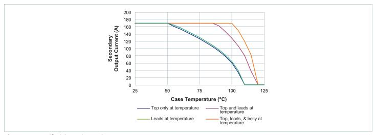
Figure 1 — Specified thermal operating area
