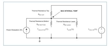
Figure 24 — Top case thermal model
