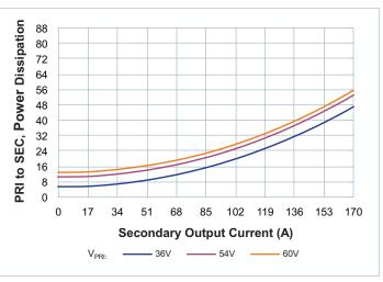
**Figure 11** — Power dissipation at  $T_{CASE} = 90$ °C
