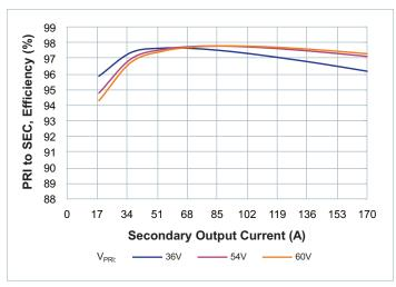
**Figure 10** — Efficiency at  $T_{CASE} = 90$ °C
