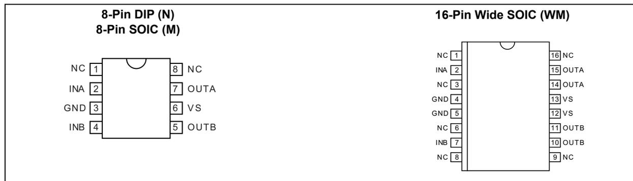
**Note:** WM Package: Duplicate GND,  $V_S$ , OUTA, and OUTB pins must be externally connected together.
