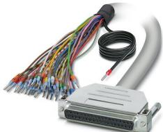
Assembled shielded round cable; connection 1: Single wires (37-position) (The wires are marked and fitted with ferrules. The braided shield is routed to a separate cable end.); connection 2: D-SUB socket strip (1x 37-position); cable length: 3 m
