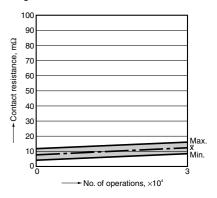
4. Electrical life test (22A 250V AC  $\cos\phi$  = 0.8 Inductive load) Sample: ALFG1PF09, ALFG1PF091, 6 pcs. Operation frequency: ON:OFF = 0.1s:10s Ambient temperature: 85°C 185°F
