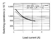
Reference: A maximum current of 0.6 A can be switched at 125 VDC ( $\cos\phi$  = 1). Maximum current of 0.2 A can be switched if L/R is 7 ms. In both cases, a life of 100,000 operations can be expected. The minimum applicable load is 1 mA at 5 VDC (P reference value).
