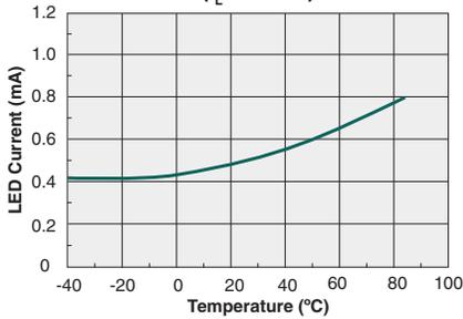
**Typical  $I_F$  for Switch Dropout vs. Temperature**
