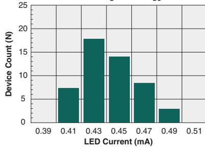
Typical  $I_F$  for Switch Dropout
