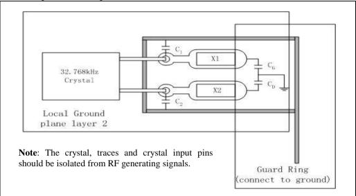
**Built-in Capacitors Specifications and Recommended External Capacitors**
