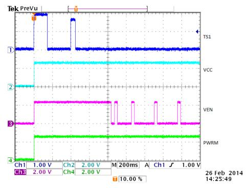
Figure 10. Valid VCC to Full FW Operation
