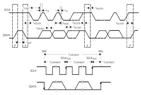
Figure 1. SMBus Timing Diagram
