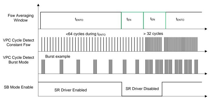
Figure 22. Standby Mode Operation
