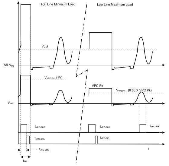
Figure 18. VPC Blanking Time Criteria
