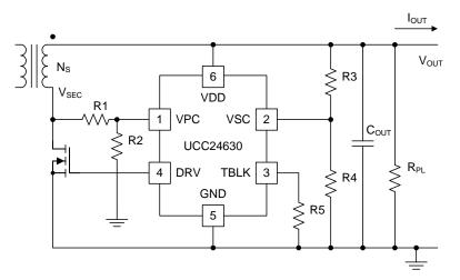
Figure 17. SR Controller Components
