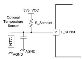
Figure 6. Negative Temperature Coefficient (NTC) Application
