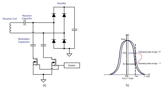
Figure 4. Receiver Capacitive Modulation Circuit
