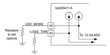
Figure 5. Option Select Pin Programming
