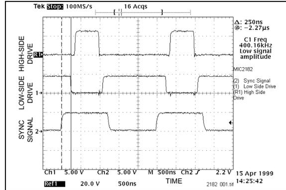
FIGURE 4-8: Sync Waveforms.
