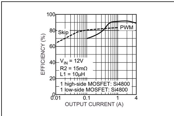
**FIGURE 2-27:** Efficiency at V<sub>IN</sub> = 12V, V<sub>OUT</sub> = 3.3V (4A Power Supply Configuration).
