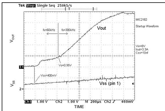
**FIGURE 4-11:** Startup Waveforms.
