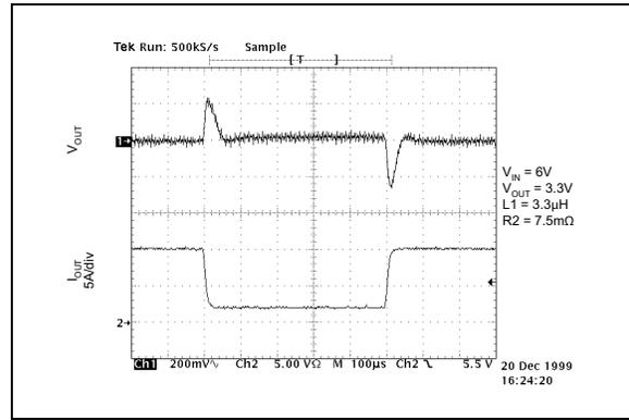
**FIGURE 2-23:** Load Transient Response (10A Power Supply Configuration).
