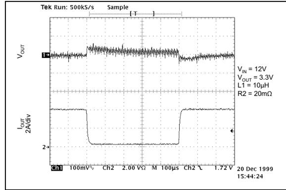
**FIGURE 2-22:** Load Transient Response (4A Power Supply Configuration).
