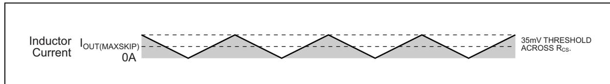
**FIGURE 4-7:** Maximum Skip-Mode-Load Inductor Current.
