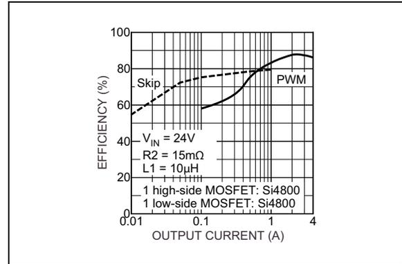
**FIGURE 2-28:** Efficiency at V<sub>IN</sub> = 24V, V<sub>OUT</sub> = 3.3V (4A Power Supply Configuration).
