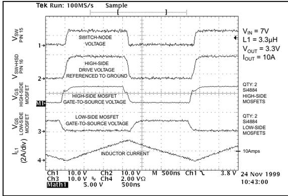
**FIGURE 2-19:** Converter Waveforms.
