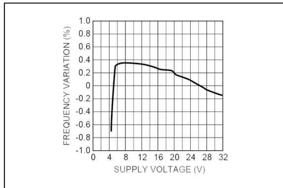
**FIGURE 2-12:** Oscillator Frequency Variation vs. Supply Voltage.
