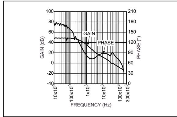
**FIGURE 2-24:** Bode Plot (4A Power Supply Configuration).
