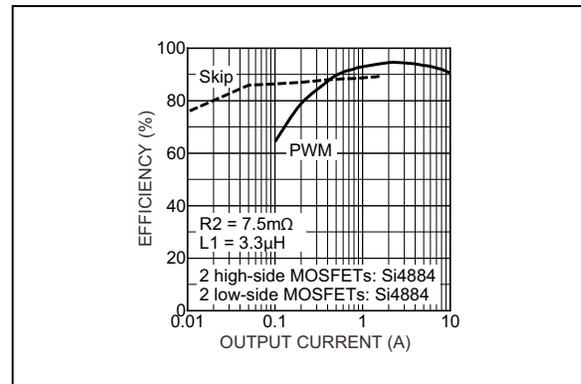
**FIGURE 2-29:** Efficiency at V<sub>IN</sub> = 5V, V<sub>OUT</sub> = 3.3V (10A Power Supply Configuration).
