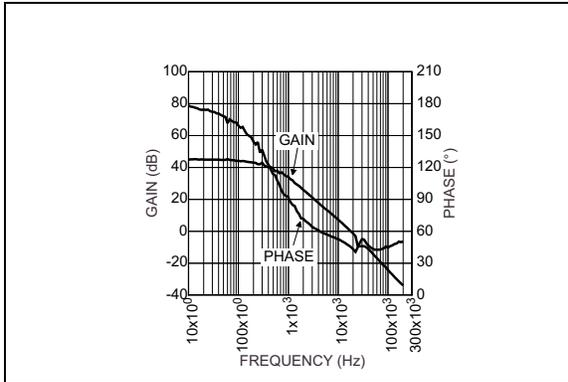
**FIGURE 2-25:** Bode Plot (10A Power Supply Configuration).
