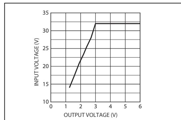
**FIGURE 4-12:** Max. Input Voltage in Forced-PWM Mode.
