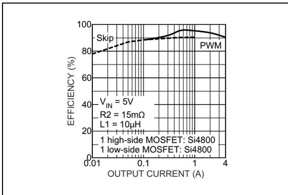
**FIGURE 2-26:** Efficiency at V<sub>IN</sub> = 5V, V<sub>OUT</sub> = 3.3V (4A Power Supply Configuration).
