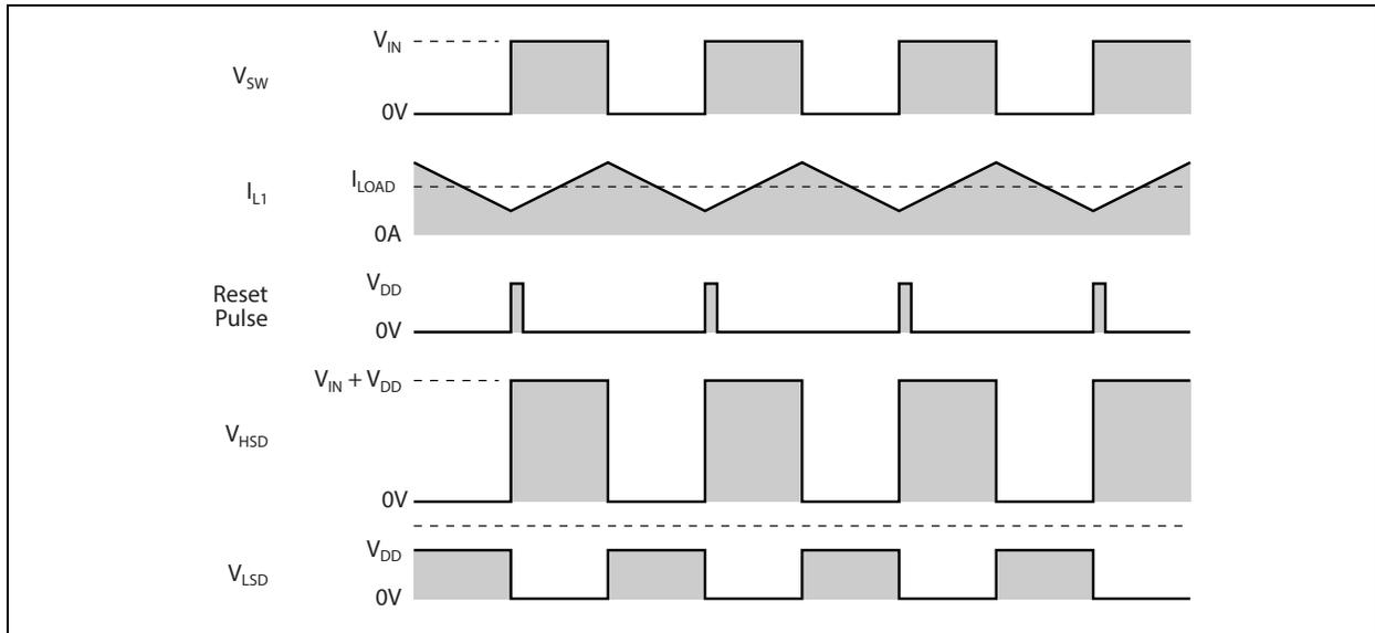
**FIGURE 4-3:** PWM-Mode Timing.
