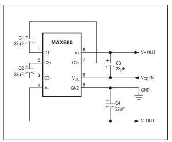
Figure 3. Positive and Negative Converter
