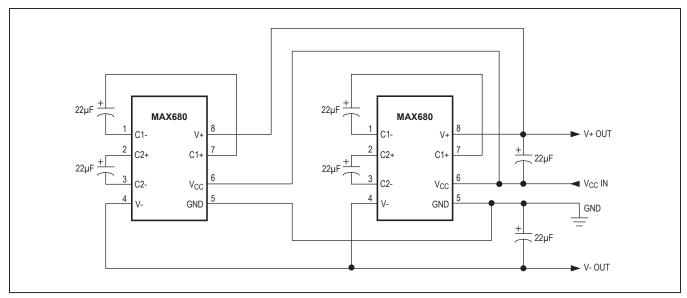
Figure 4. Paralleling MAX680s For Lower Source Resistance
