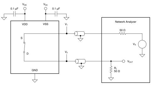
Figure 36. Bandwidth Measurement Setup
