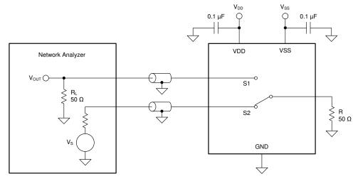
Figure 35. Channel-to-Channel Crosstalk Measurement Setup
