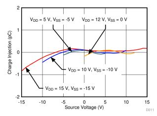
Figure 40. Source-to-Drain Charge Injection
