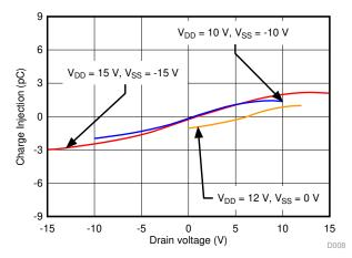
Figure 41. Drain-to-Source Charge Injection
