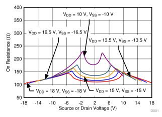
Figure 42. On-resistance vs Source or Drain Voltage
