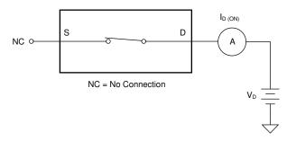
Figure 28. On-Leakage Measurement Setup
