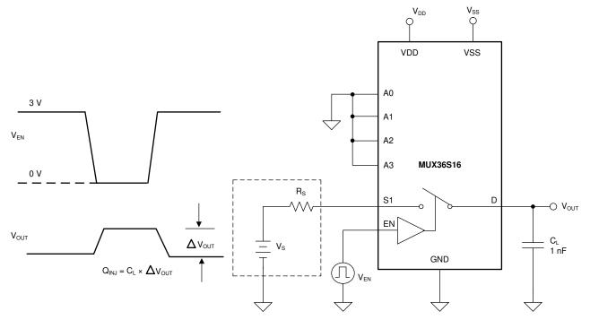
Figure 33. Charge-Injection Measurement Setup
