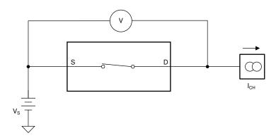
Figure 26. On-Resistance Measurement Setup
