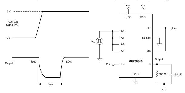
Figure 31. Break-Before-Make Delay Measurement Setup
