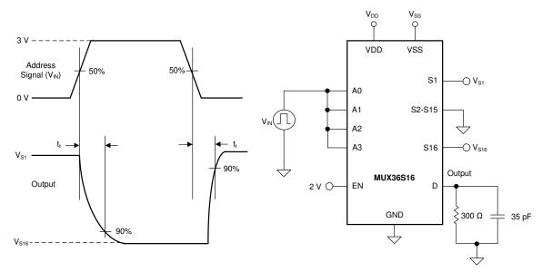
Figure 30. Transition-Time Measurement Setup
