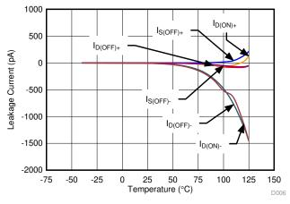
Figure 38. Leakage Current vs Temperature
