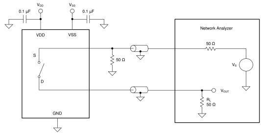
Figure 34. Off Isolation Measurement Setup
