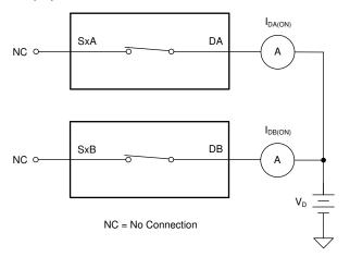
Figure 29. Differential On-Leakage Measurement Setup
