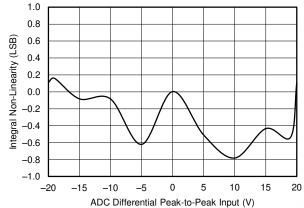
Figure 44. ADC 16-Bit Linearity Error for the Multiplexed Data-Acquisition Block
