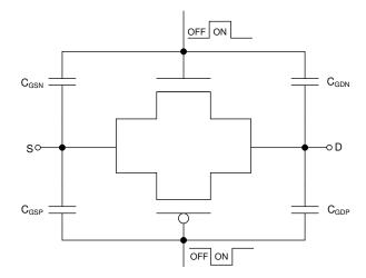
Figure 39. Transmission Gate Topology
