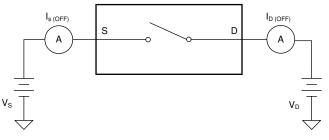
Figure 27. Off-Leakage Measurement Setup
