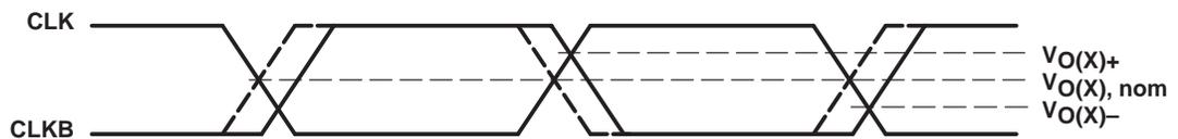
Figure 7. Crossing-Point Voltage
