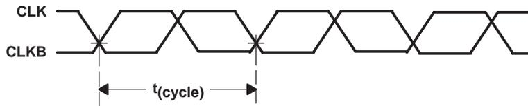
t<sub>JL</sub> = | t<sub>(cycle), max</sub> - t<sub>(cycle), min</sub> | over 10000 consecutive cycles
