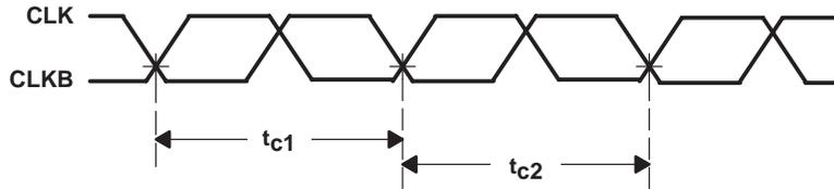
Cycle-to-cycle jitter = | t<sub>c1</sub> - t<sub>c2</sub> | over 10000 consecutive cycles
